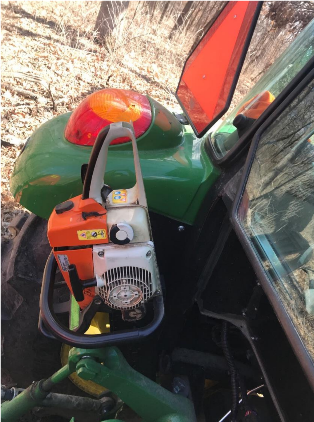
It is nice to have a chainsaw with the tractor that is mowing fire breaks. This chainsaw sits in a “Saw Haul” scabbard. Photo below is of the scabbard bolted to the fender.
